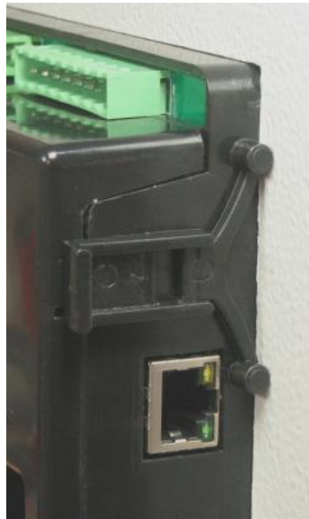
Installation of self retaining type bracket
