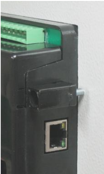
Installation of screw type bracket
