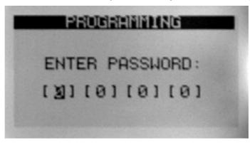
A 4 digit password must be entered using **ACK/RESET**, ▼ and ▶ buttons.
