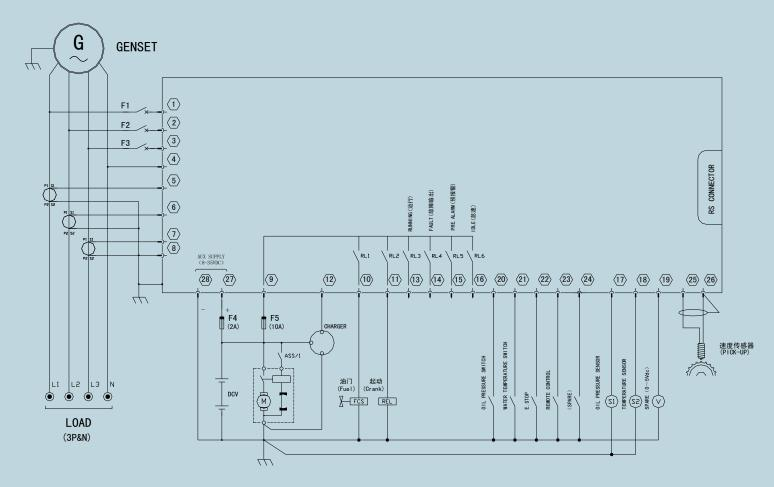
NOTE: CATHODE OF THE BATTERY AND SHELL OF THE CONTROLLER MUST BE GRANDED PROPERLY!
