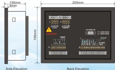
Front Elevation Side Elevation
