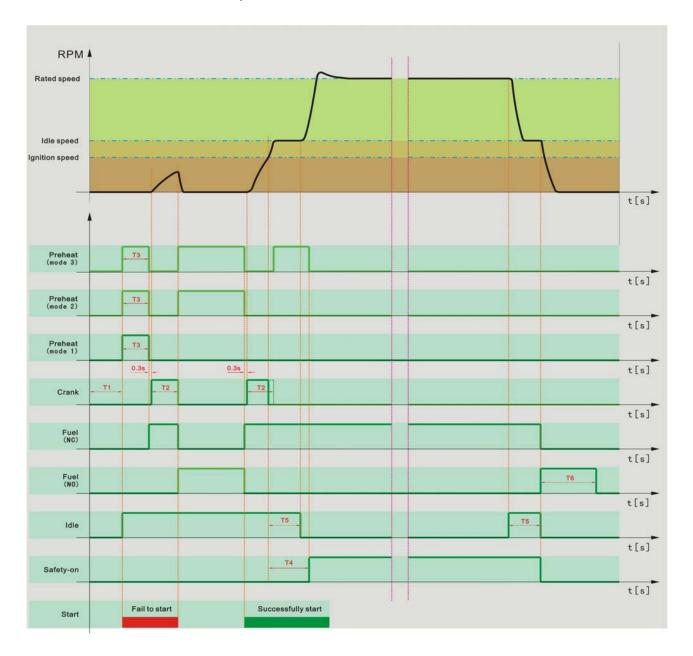
T1— start delay T4—safety-on delay T2— crank time T5— idle time
