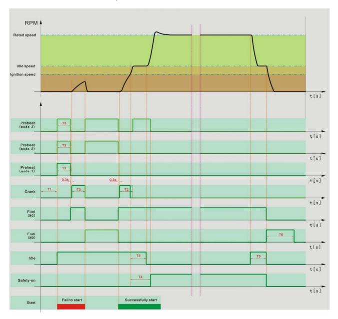
T1 - start delay T4 — safety-on delay
