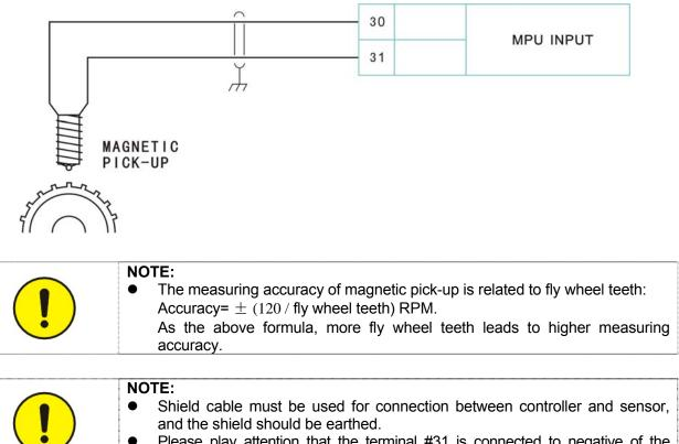
• Please play attention that the terminal #31 is connected to negative of the power supply inside the controller.
