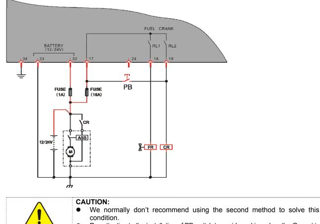
Pay attention to the installation of PB switch to avoid cranking when the Genset is running.
