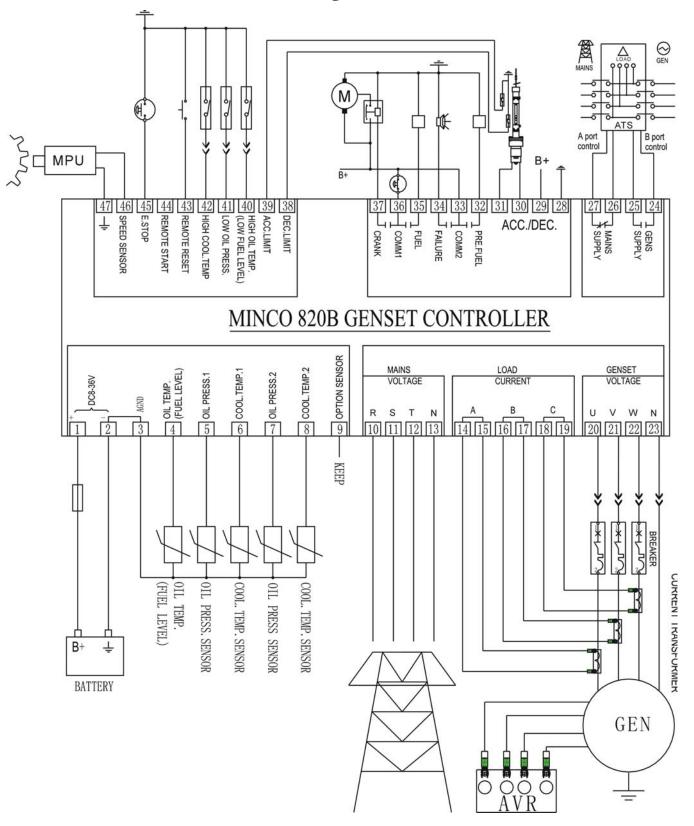
Minco820B Outside wire connection drawing(Mechanical speed control)
