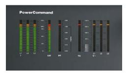
The PowerCommand control can be equipped with an analog AC metering panel that simultaneously displays 3-phase line to line AC volts and current, kW, power factor, and frequency.
