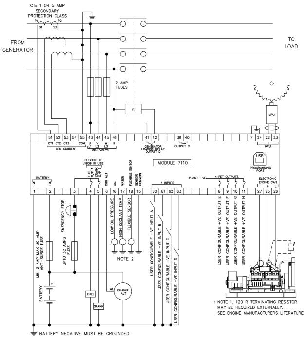
TERMINALS SUITABLE FOR 22-16 AWG (0.6mm - 1.3mm ) FIELD WIRING
