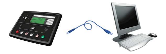
ANOTE:- The DC supply must be connected to the module for configuration by PC.
