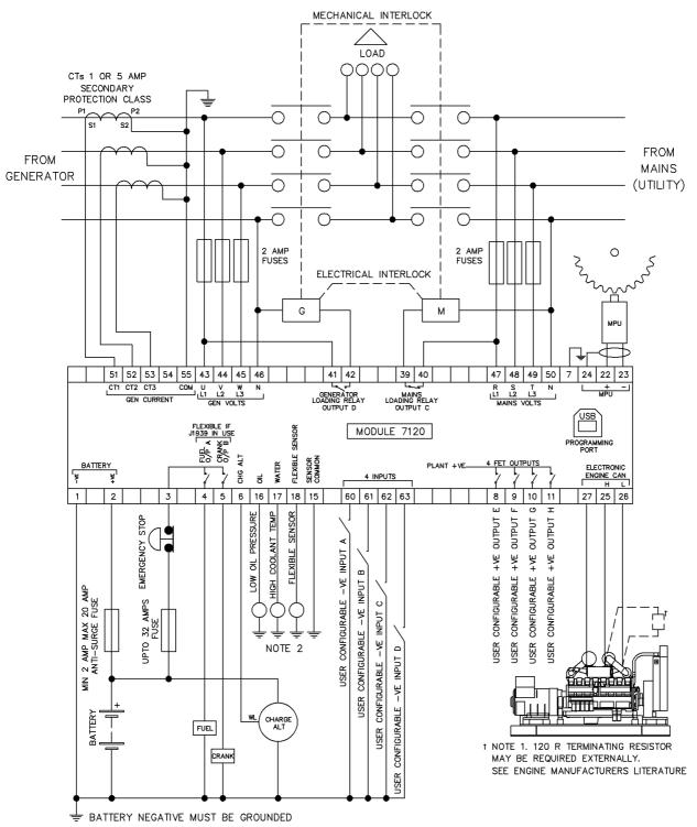
TERMINALS SUITABLE FOR 22-16 AWG (0.6mm - 1.3mm ) FIELD WIRING
