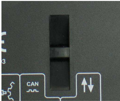
Cable tie fixing point
